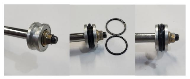
9. Lubricate the O-Ring on the end cap and T-Seal on the piston then carefully install the assembly into the main housing being sure not to cut the seals during this. Once the piston is inserted it becomes important to align the end cap with the hole in the housing before pushing it in. Once installed it will be difficult to rotate the cap into position if it is far off. Temporarily install one of the end fittings to ensure the cap doesn't move out of position.
