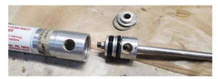
6. Using 9/32 and 5/16 wrenches, remove the nut retaining the piston from the end of the shaft. Remove the piston and hardware from the shaft. Discard the old sealing washer and AN960-416 washer.
