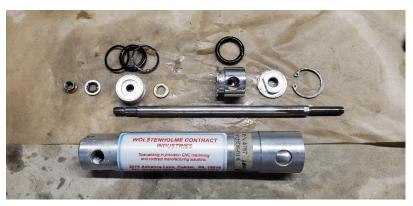
Note: Some 4787 actuators were provided with a square cross section O-Ring instead of the U-cup seal. It is unclear why this was done, possibly due to shortages or cost of the proper U-cup design. While these may work, they are not ideal under the high pressures these actuators are subject to. The kit replaces these with U-cup seals intentionally to improve sealing and reduce wear.
