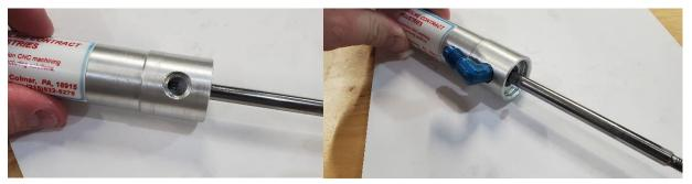
10. Reinstall the end cap retainer. Reinstall the snap ring with the "sharp" edge facing away from the retainer plate. Be sure to orient the snap ring so that the legs are 180deg away from the clearance section of the retainer, this provides extra security that the ring will not come out. This is done by rotating it with the snap ring pliers after it is installed as shown below.
