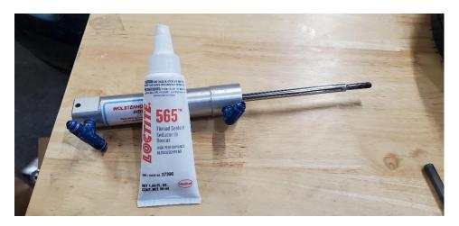
12. Reinstall the hardware onto the end of the cylinder, reinstall the cylinder into the plane. Leak and function test prior to flight.
