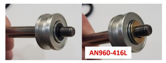
Note: The AN960-416L washer was not originally used by Lancair and is not needed, however it does reduce the opportunity for the sealing washer to become damaged during assembly due to the friction between the nut and rubber.
