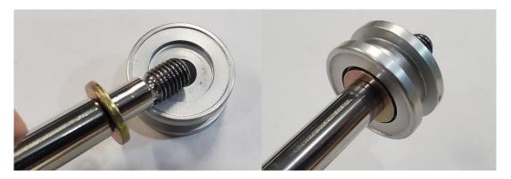
6. After lubricating, install the sealing washer onto the end of the shaft. Inspect the AN960-416L washer for burrs and place the more "sharp" side toward the sealing washer. Again, this washer should be lapped flat if required to remove any burrs.
