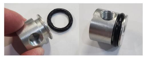
2. Lubricate and install the U-Cup into the front of the end cap. The U-Cup should be oriented as shown, with the lip facing inside of the cylinder assembly and the flat part on the outside.
