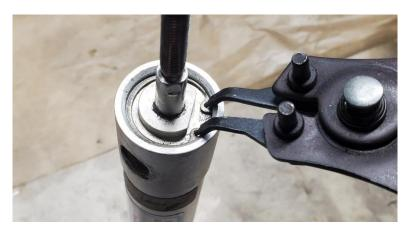
4. Remove the retaining plate. Check the snap ring groove for any burrs that could cause damage to the end cap or piston when removed.
