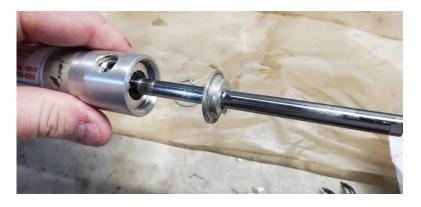
5. Using a firm grip, grab the end of the shaft and pull the shaft assembly out of the housing.
