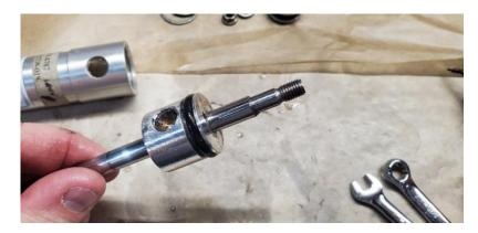
8. Carefully remove the U-Cup seal and O-ring from the aluminum end cap. Remove the T-seal from the piston. Discard these components. Do not use metal picks of any kind to remove these seals.
