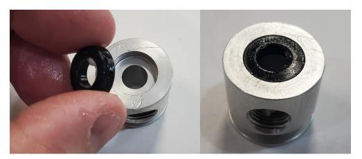
3. Lubricate and install the end cap onto the shaft by sliding it on from the piston end.
